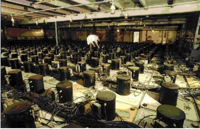
FIGURE 2.8 View of one of four horizontal arrays of the Baksan scintillation telescope. Source: Courtesy of A.V. Voevodsky.
