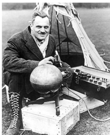
Figure 37. Arthur Compton near ionization chamber, developed by him for eight cosmic ray expeditions worked in 1932.
